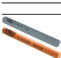
These files are used in particular for machining tools in the wood and machine construction industries. Thanks to the varying grit sizes you can select the perfect tool for your application. Silicon carbide files are primarily used for tungsten carbide or tungsten carbide tipped tools and are grey-green in colour. Orange is used primarily for all types of steels and stainless steel.
