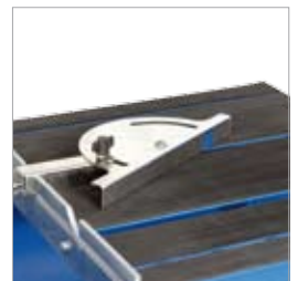
Included angle stop for cuts from 30° to 90°
